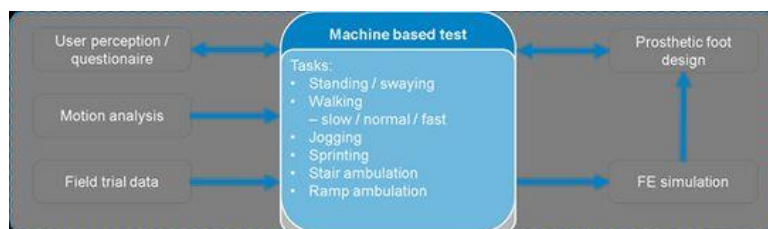
Figure 1. Overview of the task specific tests investigated in relation to the user input and optimization output.
