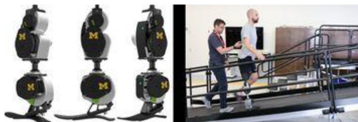
Figure 1. (Left) Rendering of the OSL. (Right) Patient walking up a ramp using the OSL.
