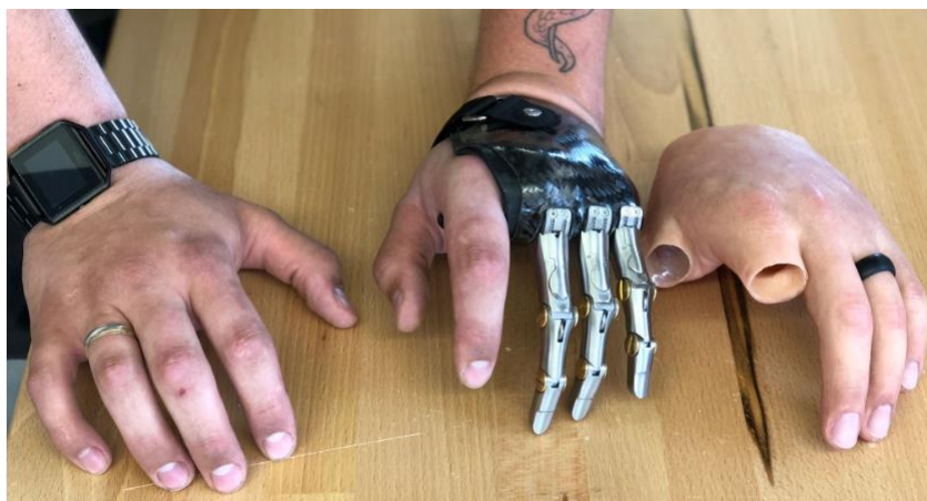
Figure 1. A partial hand amputee displaying the intact hand (left), ratcheting cosmetic prosthetic finger (center), and cosmetic covering (right)..
